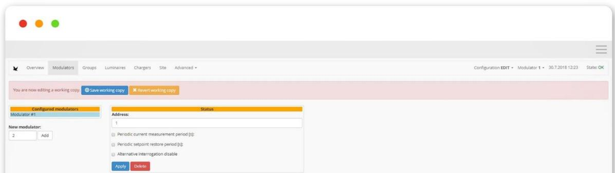
Once added, a window appears with a list of configured modulators "Configured modulators", „Status“ with the status of modulator, Actual values of the measured quantities. You can send
